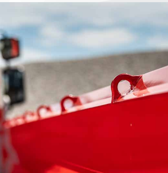
Side and front wall lashing eyes also for transporters and light 2-axle vehicles
