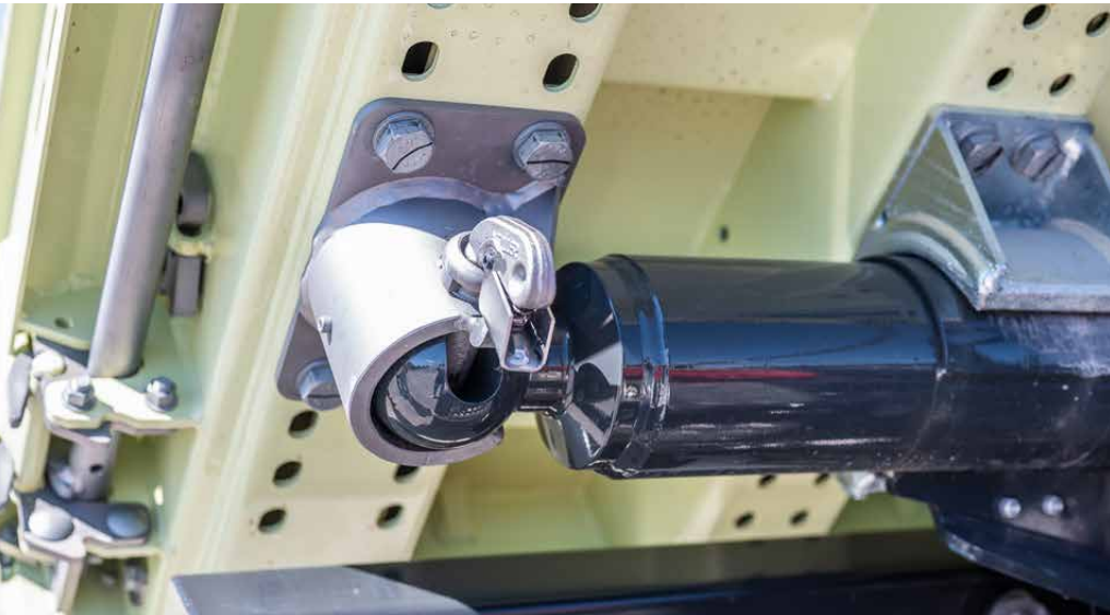
NEW: Ball-type tipping parts for one-hand operation
