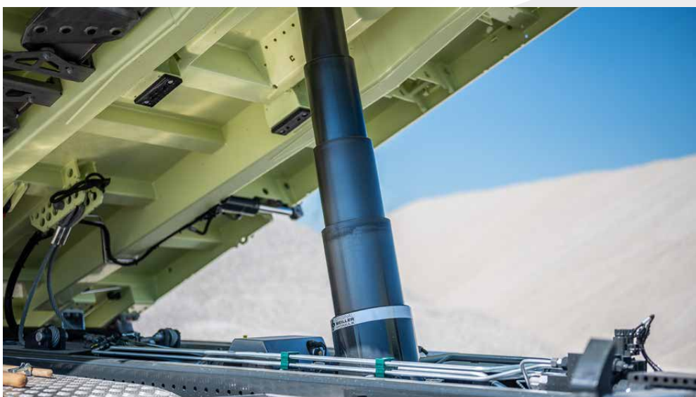
NEW: Only one hydraulic telescopic cylinder on the 4-axle vehicle
