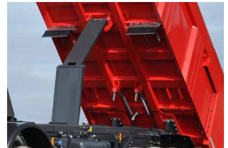
MEILLER scissor tipping stabiliser gives safety when tipping.
