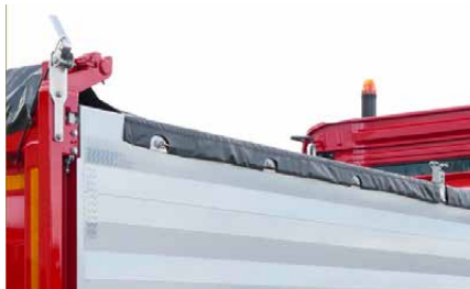
An eccentric bearing on the top belt of the tipper body allows the retensioning of the side roller tarpaulin.
