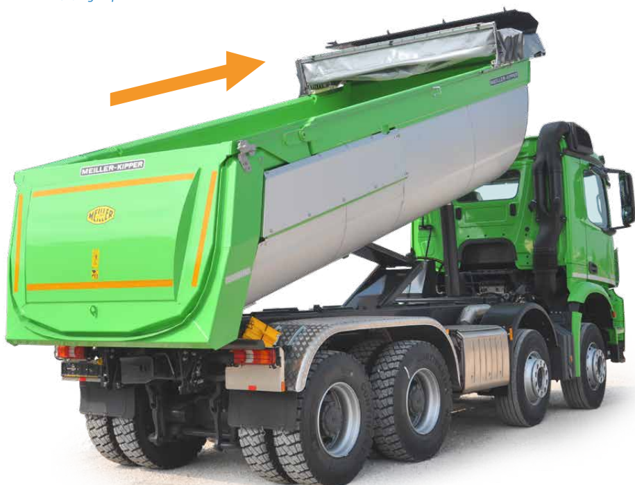
MEILLER rear tipper with electrical sliding tarpaulin.
