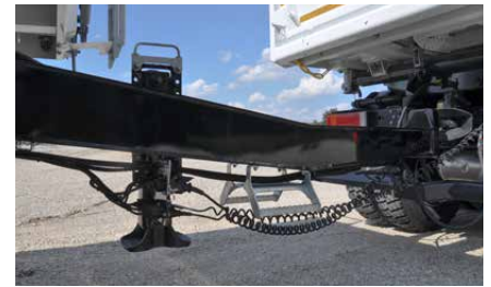
The climb-over on the tow bar with handle on the stabilising leg facilitates the opening and closing of the side roller tarpaulin on the centre-axle trailer.
